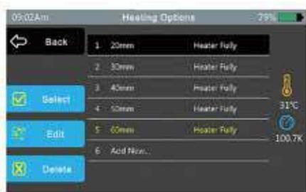
Select the required heating mode, and press the button (the yellow script is the currently selected heating mode)
