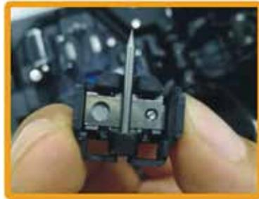
Remove the old electrode, loosen the screw attached to the electrode cover, and remove the old electrode rod.
