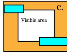
The fiber end face is above or below the visible area of the lens and cannot be found automatically.
