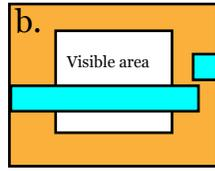
The fiber end face is beyond the visible area of the lens.
